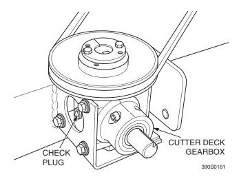
Figure 7-8. Cutter Deck Gearbox
